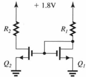
$$\text{From Ex: 5.9, } V_{GS} = 0.8 \text{ V, } V_{in} = 0.5 \text{ V,}$$
