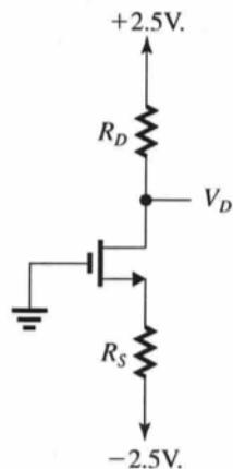
$$V_t = 1 \text{ V}, k'_n = 60 \text{ } \mu\text{A/V}^2$$
